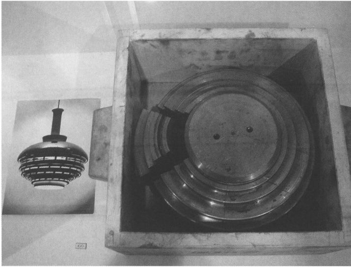
Fig. 15. Alvar Aalto, Artek lamp no. A335, with the original jig from Valaistustyö Ky (Author)
